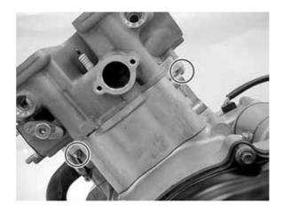
Remove the bolt and then remove the cylinder head.
