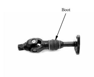
Inspect the splines of universal joint for wear or damage.
