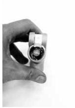
Check the spring and piston for scratch, corrosion or other abnormal condition.
