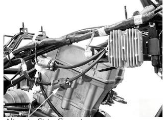
**Alternator Stator Connectors**
