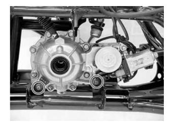
Install the front propeller shaft. Install and tighten the three new bolts to specified torque.
