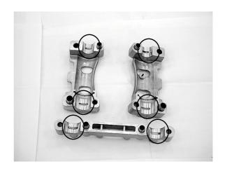
Apply molybdenum disulfide oil to the camshaft journals of the cylinder head.
