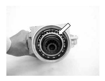
Check the outer race play and smooth rotation of the bearing by hand while it is on the front drive.
