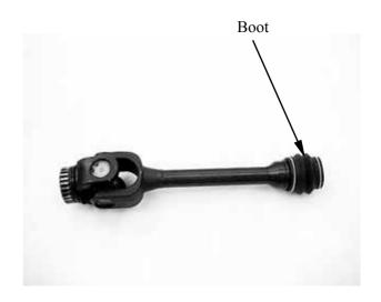
Inspect the splines of universal joint for wear or damage.
