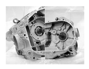
Remove the fifteen bolts from right crankcase.
