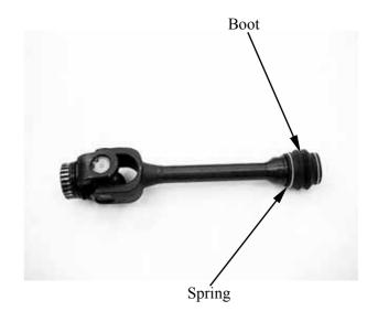
Remove the snap rings from the universal joint.
