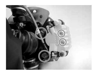
Compress the brake caliper holder and remove brake pads.
