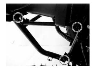
Remove the three mounting bolts from front carrier left side.
