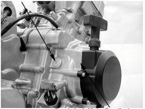
Crankshaft Hole Cap/O-ring
