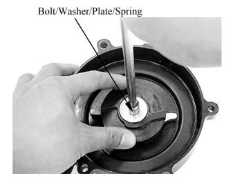
Remove the reel, then remove the coil spring.
