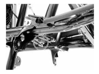
Remove the collar and dust seal.
