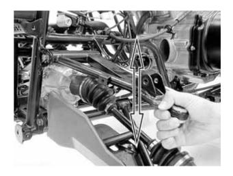
Check the front lower arm bracket of the frame.
