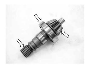
Check the cover and case bearings for wear or damage.
