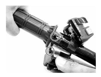
Place the right and left brake master cylinder on the handlebar and install the master cylinder holder with the "UP" mark facing up, aligning the punch mark on the handlebar with the holder joint seam. First tighten the upper bolt and then tighten the lower blot.
