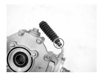
Turn the pinion gear and check that the gear turns smoothly and quietly without binding.
