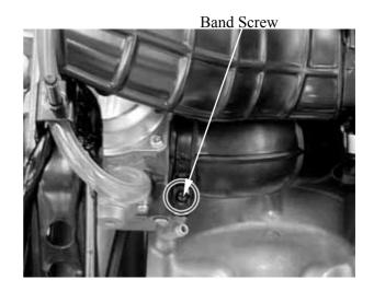
Remove the clip and disconnect the crankcase breather hose from the crankcase. Remove the mounting bolts and then remove the air cleaner housing from the carburetor and the intake duct.
