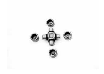
Insert the universal joint to the new bearing and check the play by turning the universal joint, as shown.
