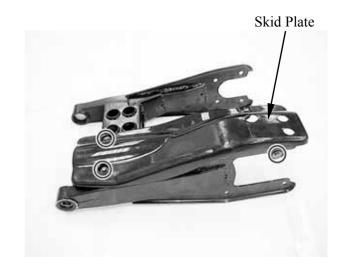
Inspect the swing arm for distortion or damage.
