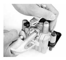
Inspect the caliper cylinder wall and piston surface for scratch, corrosion or other damages.
