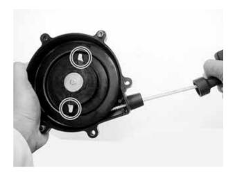
Inspect the rope, reel and drive pawl for wear or damage.
