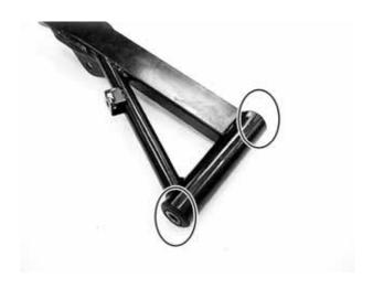
Inspect the front lower arm. Cracks/bends/damage →Replace.
