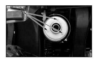
2. Remove the spark arrester (2) and the gasket (3) from the muffler.
