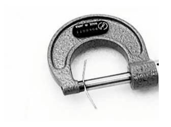
Select the proper size of shim(s) from the right chart, according as the compressed solder thickness.
