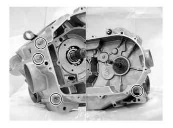
Install the stopper, spring, washer and plug. Tighten the stopper plug to the specified torque.
