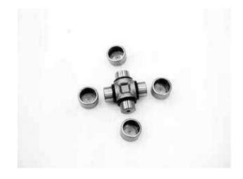
Insert the universal joint to the new bearing and check the play by turning the universal joint, as shown.
