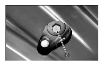
6. Clean the oil strainer with solvent. Inspect the O-ring and replace if damaged. Reinstall the O-ring, oil strainer, compression spring and oil filter cap. Tighten the oil filter cap to specification.
