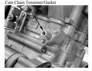
Remove the two bolts and cam chain guide.
