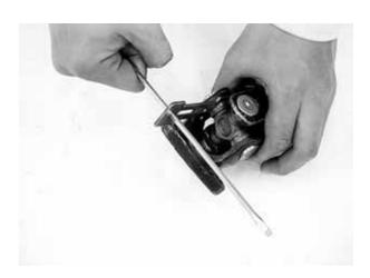
Remove the bearings by tapping the universal joint with a copper hammer.
