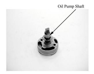
Remove the screw and oil pump cover.
