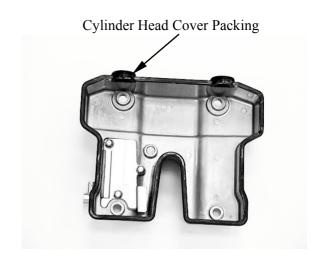
Install the cylinder head cover. Install and tighten the four bolts/rubber washers to the specified torque in a crisscross pattern.
