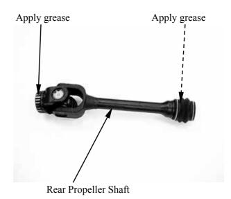
Install the rear propeller shaft into the engine assembly.
