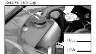
Fill the system with the recommended coolant through the filler opening up to the filler neck.
