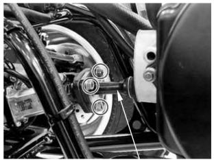
Front Propeller Shaft
