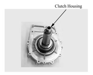
Remove the oil seal, then remove the bearing.
