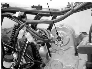
Gear Indicator Light Switch Connector
