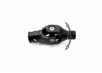
Apply lightweight lithium-soap base grease to the shaft splines and inner.
