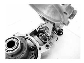
Apply three bond: 1215 to the case bolts and tighten them to the specified torque in a crisscross pattern in 2 or 3 steps.
