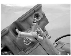
Water Joint/Gasket/Water Stop Collar
