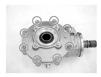
Pry the cover at the prying point using a screwdriver.
