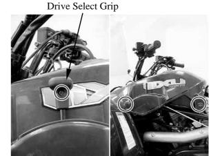
Remove the two fasteners from fuel tank cover right side.
