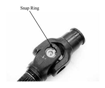
After reassembling the universal joint, check the joint movement smoothly. If a large resistance is felt to movement, tap the bearing with a plastic mallet lightly.
