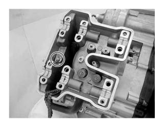
Remove the dowel pins and gasket.
