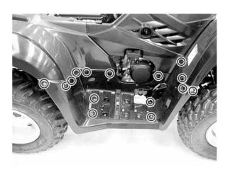
Remove the eight fasteners, two screws/nuts and four bolts, then remove the left footboard.
