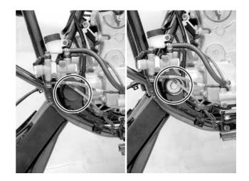
Remove the bolt and band, then remove the rear brake fluid hoses from swing arm.
