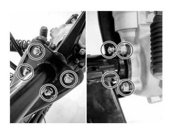
Remove the left rear axle housing from the rear drive case.
