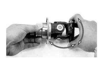
Before install the universal joint yoke assembly, place the snap ring between the shifting sleeve and splines of universal joint.
