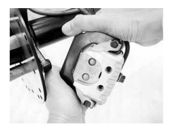
A wear indicator is provided on each brake. The indicators allows checking of brake pads wear. Check the position of the indicator.
