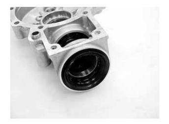
Check the right gear case bearing for wear or damage.
