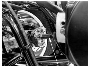
Front Propeller Shaft
