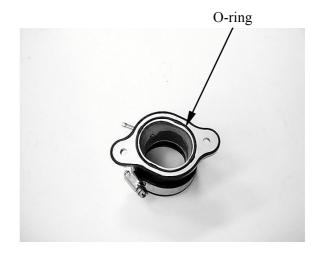
Install the intake pipe and tighten the two bolts securely.
