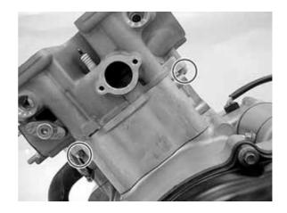
Install the water stop collar, gasket and water joint.
