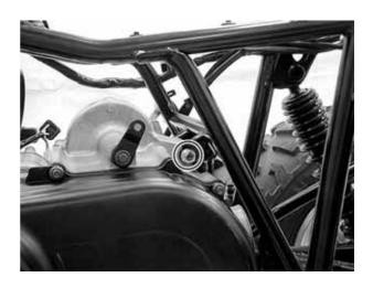
Rise the engine front side and move the engine forward, then remove the engine from the frame by disengaging the rear drive gear case.
