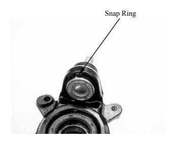
Remove the knuckle end by using the appropriate collar.
