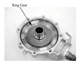
Install the removed right shim to the ring gear.
