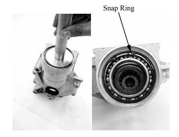
Install the new oil seal into the right gear case.
