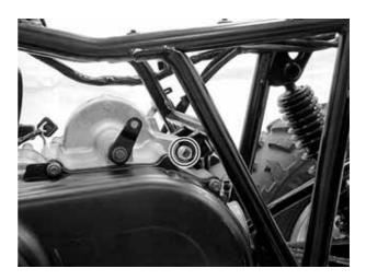
Lower Engine Mounting Bolt/Nut
