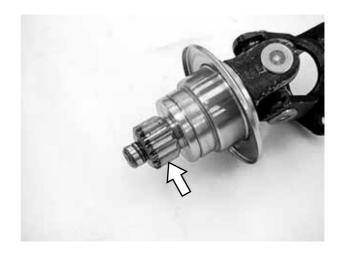
Inspect the universal joint, wear and damage.
