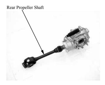
Install the rear propeller shaft and rear drive assembly to the engine and right rear axle housing.
