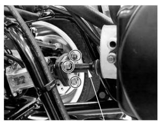
Front Propeller Shaft
