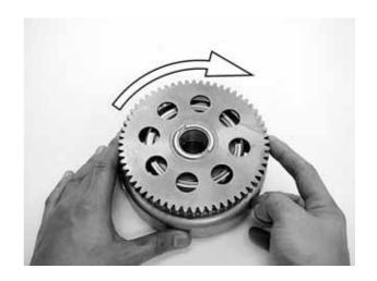
Check the starter driven gear teeth for wear or damage.
